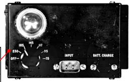
The 12V accumulator of a RS-13 station was charged by a separate AC powered charger unit.
