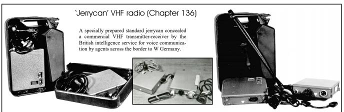
The hitherto unknown make and type of a commercial VHF portable transmitter-receiver originally was carried on the body using a small harness.
